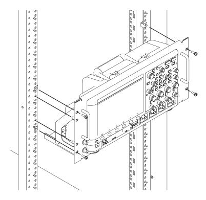
**3** Fasten the support shelf to the rack cabinet using four 10-32 dress screws.
