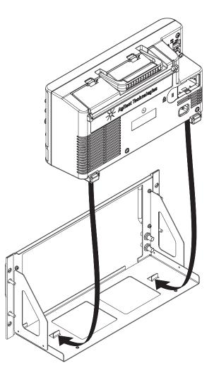
**2** Push the oscilloscope fully forward on the support shelf assembly.
